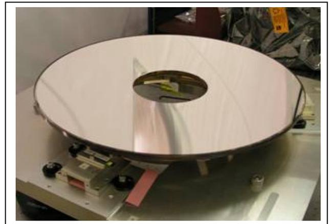
**Figure 3: Primary Mirror in bonding fixture**
