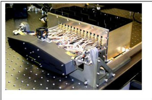
**Figure 10: Focal Plane Assembly with filter cover in place**
