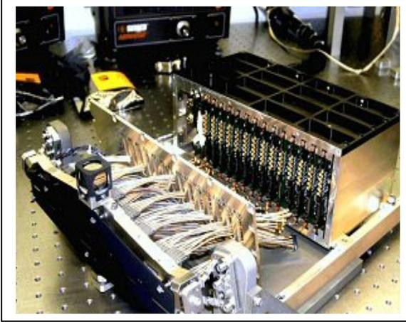
**Figure 8: Focal Plane Assembly about to be mounted to Focal Plane Electronics**
