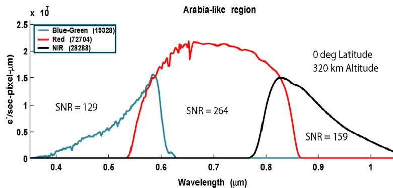
Figure 12: Signal in Electrons as a Function of Wavelength for a Bright Region of Mars
