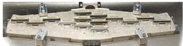
**Figure 6: 14 CCDs mounted to FPA substrate**
