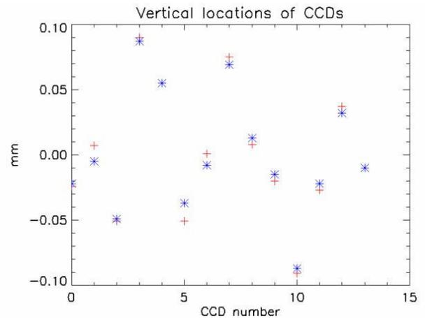
**Figure 5: Measurements of CCD vertical position on focal plane substrate. Left +, and right \* side fiducials**
