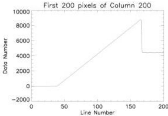
**Figure 11: Example of the first 200 lines of a column from a flat field image. First 20 lines are reverse clocked, the next 20 lines are under the mask and the next 128 lines are actual image lines contaminated by reverse clocking.**
