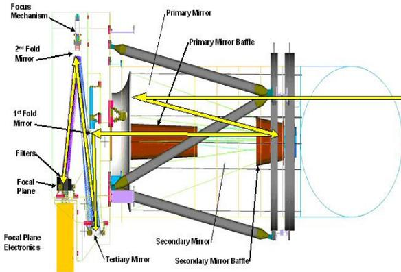
**Figure 2: Camera optical path optimized for low mass**
