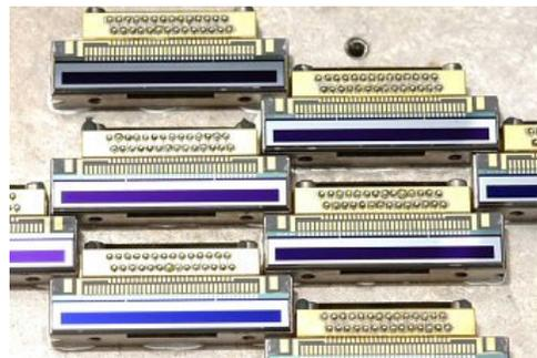
**Figure 7: Mounting of center 6 CCDs, showing custom headers for wirebonds to buffer amplifier boards**
