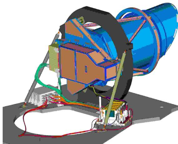
**Figure 1: HiRISE imager assembly mounted to spacecraft support ring. The two electronics boxes house the instrument controller and power supply.**
