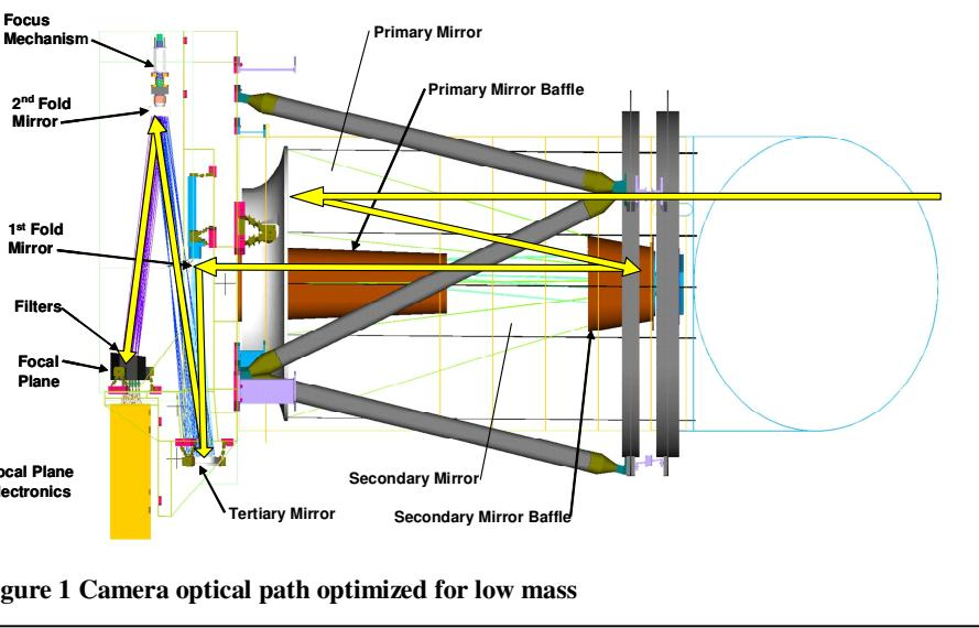
Figure 1 Camera optical path optimized for low mass
