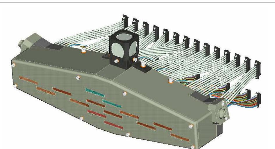
Figure 3 HiRISE Focal Plane Assembly
